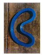
[11] The photograph that appears below shows how the beginning of the indentation to form the C-shape looks on a slightly longer piece of pipe.
